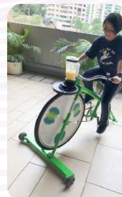
活動擺放環保單車，讓同學一邊踏單車，一邊利用產生的電能推動攪拌機，製作出美味的菠蘿沙冰。 A specially-designed bicycle is set up for students to ride and make delicious pineapple smoothie, as electricity is generated to provide power for the blender up top.
